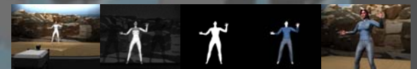
The pipeline simulated: Actor wearing white garment - IR image - Mask - Virtual clothes - The final result
